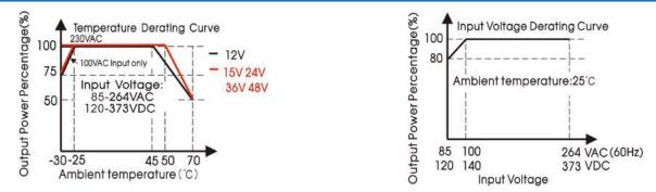
Note: ①Input voltage reduction is required on the basis of temperature reduction for the input voltage is 85 - 100VAC/120 - 140VDC; ②This product is suitable for applications using natural air cooling; for applications in closed environment please consult SCHMID-M FAE.
